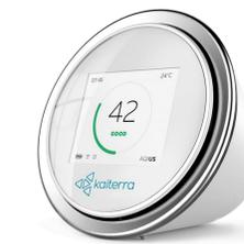
Fig. 3: A Kaiterra Laser Egg 2, used in the study to monitor PM<sub>2.5</sub> levels over time.
