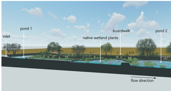
Figure 27: longitudinal section of constructed wetland
