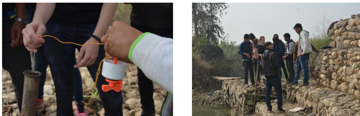
Figure 1 and 2: Action Lab team teaching the students how to deploy the Levellogger into the pipe well connected to the gabion wall
