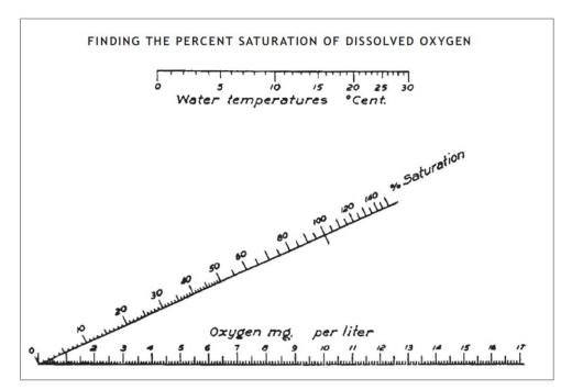
To read this chart, use a straight edge. Place the straight edge on the mg/L of oxygen you have determined for your site, then place the other end of the straight edge on the water temperature you have measured. The point where the straight line passes through the line labeled "% Saturation" is your percent saturation. Diagram reprinted from M.K. Mitchell and W.B. Stapp, *Field Manual for Water Quality Monitoring*
